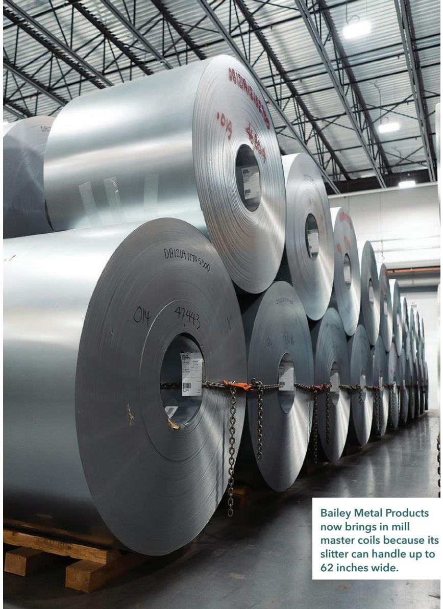
Bailey Metal Products now brings in mill master coils because its slitter can handle up to 62 inches wide.
