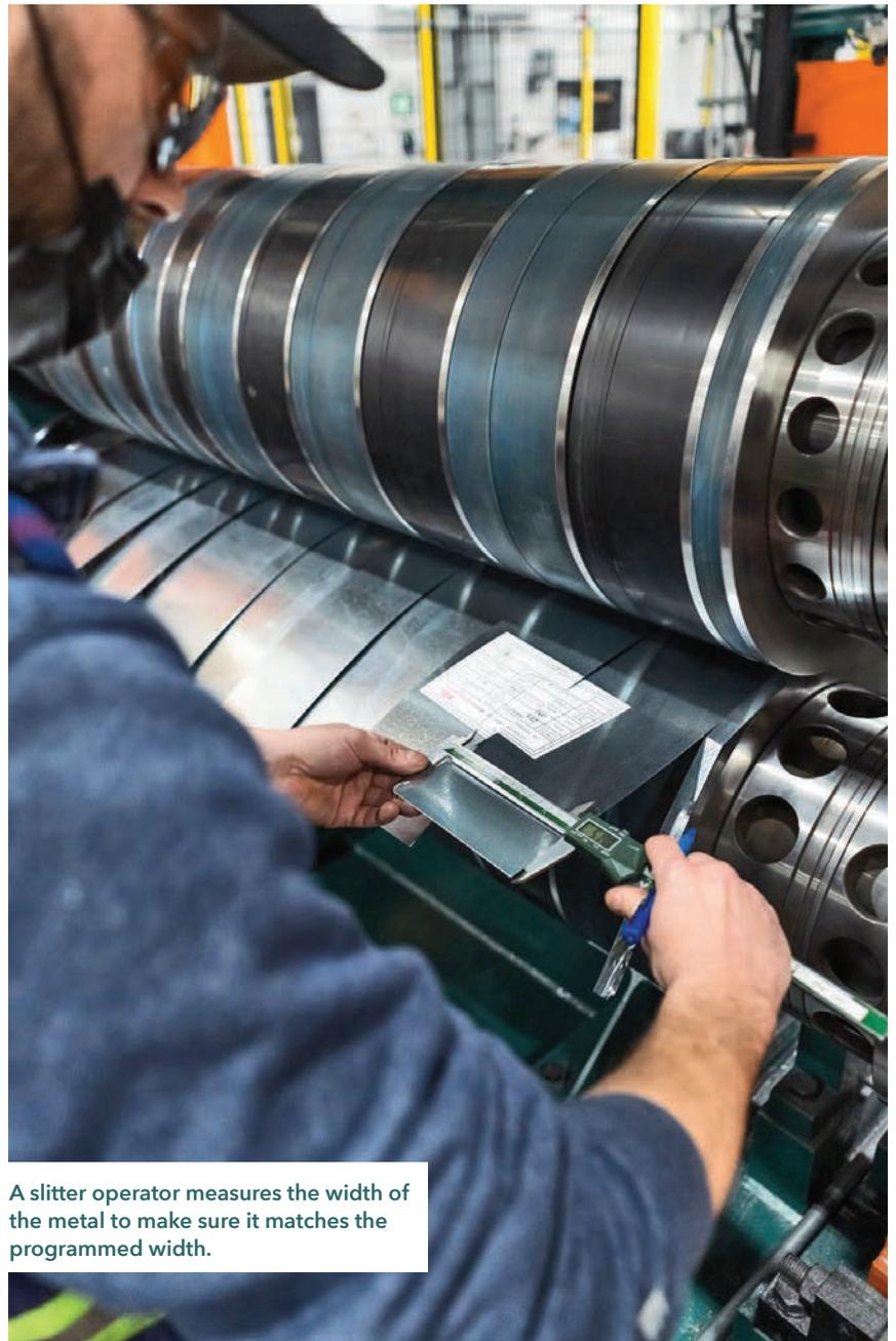
A slitter operator measures the width of the metal to make sure it matches the programmed width.
